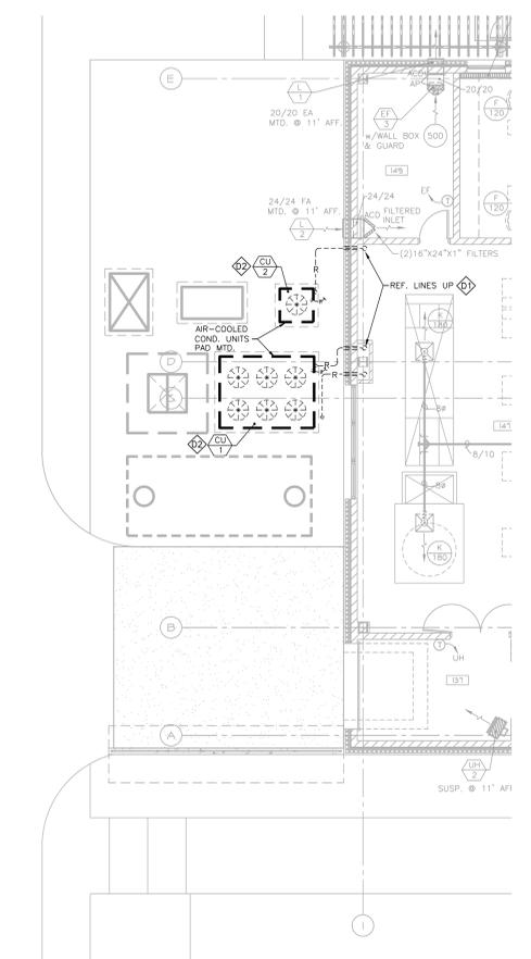
**1 PARTIAL FIRST FLOOR - HVAC DEMOLITION PLAN**
